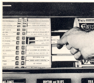
Title Strips. Each half of revolving drum shifts right or left to permit ease of removing and inserting title strips.
